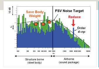
A comparison of EV- and ICE-powered class A/B car concept to enable target setting.
