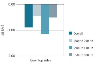
Reinforcing the cowl top connection to the A-pillar highlighted above combined with gage reductions on the surrounding panels resulted in an overall sound pressure level reduction together with a 1.4-kg weight saving (right).
